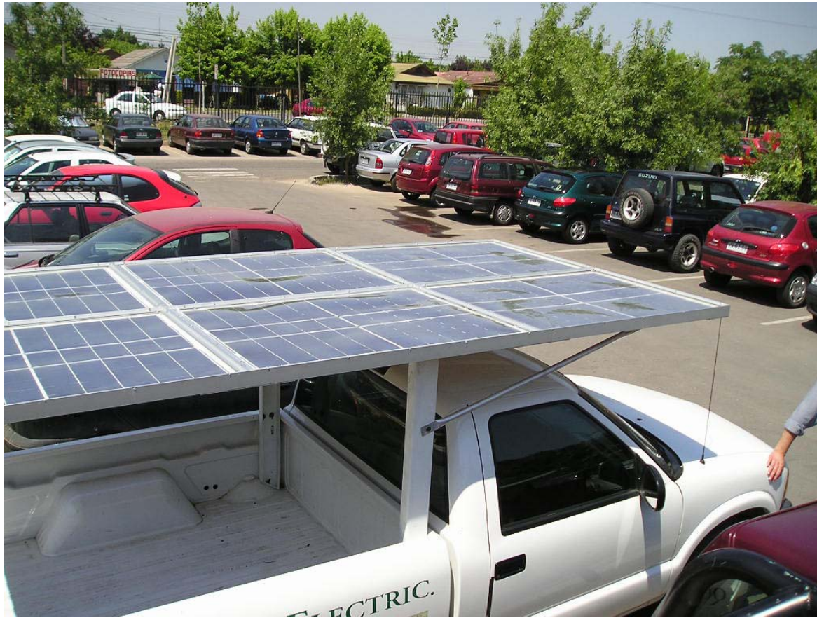
Figure 3: EV with 6 Solar Panels Installed on the Roof.
