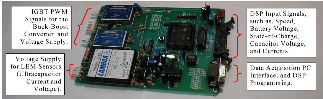
Fig. 7. DSP control circuit.
